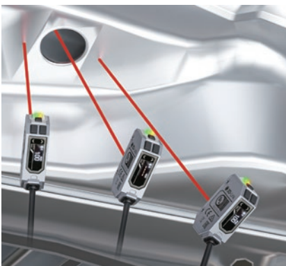
Parts identification using hole positions
