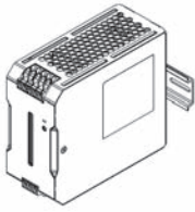
(C) Side mounting only for 15 W
