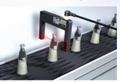
**BGL002T** BGL 80A-009-S49 20A-009-S49 Ordering code Part number Switching output PNP NPN NC/NO selectable Switching type Wiring M8 connector, 3-pin Fork opening 80 mm 120 mm Light type Laser Switching frequency 5000 Hz Degree of protection IP 67 Housing material Gd-Zn Optical surface Glass
