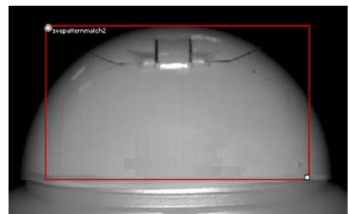
Fig. 6-4b Pattern detection of a shampoo bottle seal: NOK
