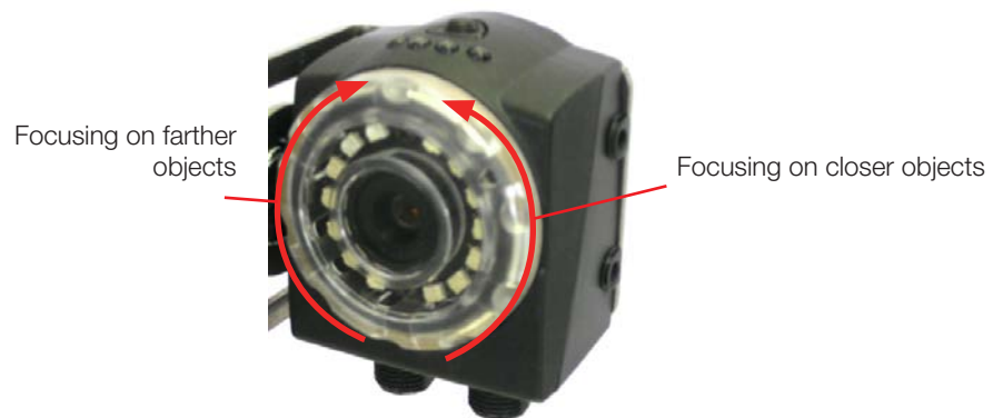
Fig. 5-1: Setting the focus
