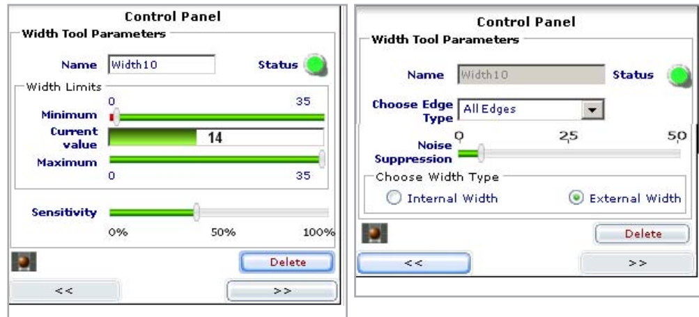
Fig. 6-6: Control Panel for Width, page 1 and page 1
