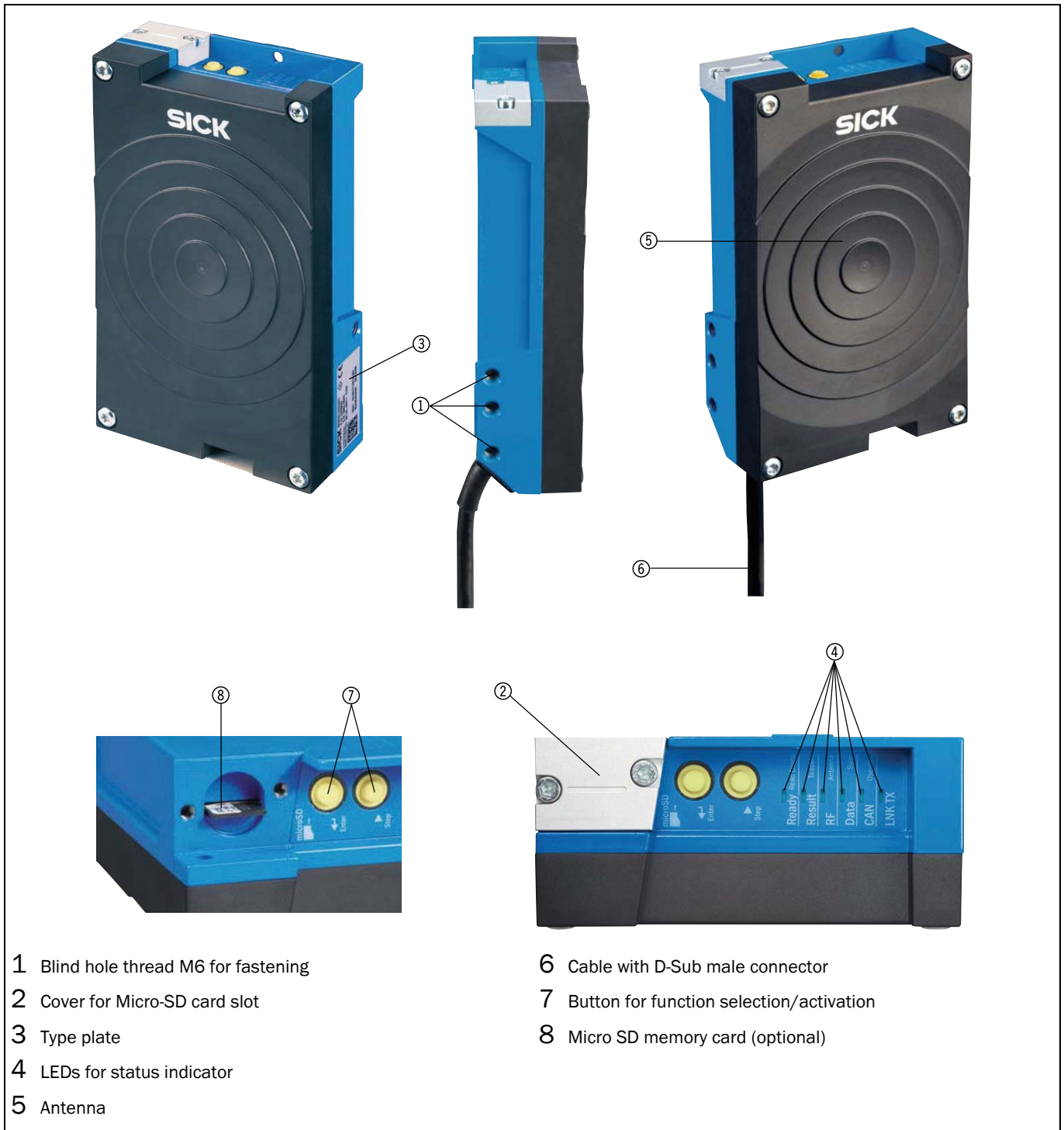
Fig. 4-1: Serial version: Device view of the RFH620-1000001
