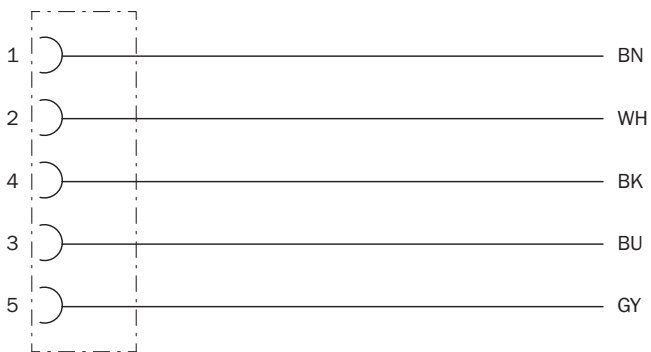
Contact assignment of the M12 female connector
