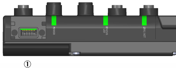
Figure 21: DIP switch on the fieldbus module
