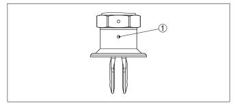
Fig. 7: Marking on the welded socket
