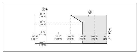
Fig. 26: Ambient temperature - Process temperature
