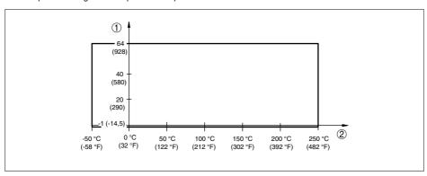
Fig. 27: Process temperature - Process pressure with switch position 0.7 g/cm<sup>3</sup> (mode switch)
