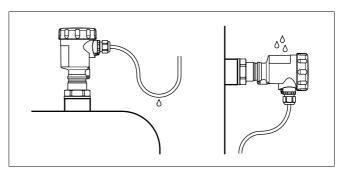
Fig. 6: Measures against moisture penetration
