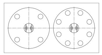
Fig. 5: Fork position with flange versions
