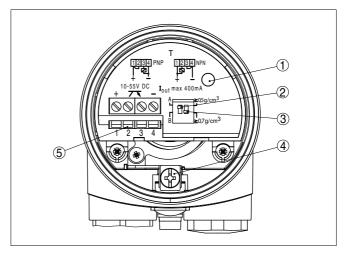
Fig. 11: Electronics and connection compartment, single chamber housing
