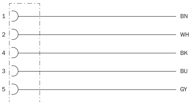
Contact assignment of the M12 female connector
