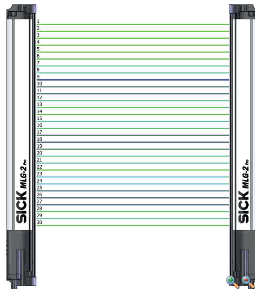
Figure 68: Beams highlighted in color in the simulation
