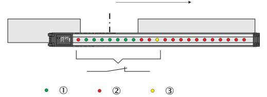
Figure 117: Classification of the hole position - smaller than or equal to hole center
