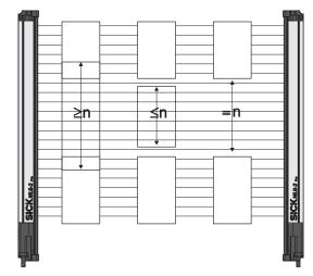
Figure 106: Hole detection/hole size
