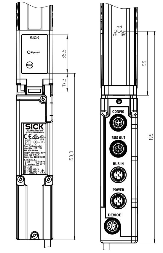
Figure 152: Dimensional drawing 1 MLG-2 fieldbus module
