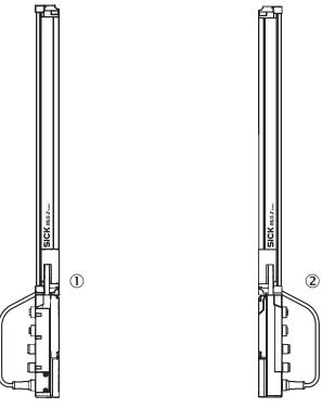
Figure 40: Mounting directions of the fieldbus module
