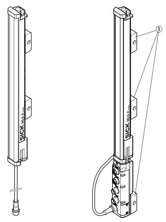
Figure 36: QuickFix bracket for the fieldbus module
