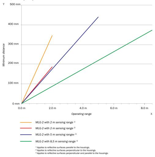
Figure 33: Graph, minimum distance from reflective surfaces
