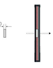
Figure 14: Minimum detectable object length
