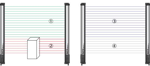
Figure 71: Example of the blanking of blocked beams
