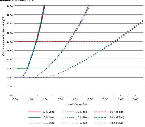
Figure 150: Minimum detectable absorption required for devices with 2 m, 5 m and 8.5 m sensing range
