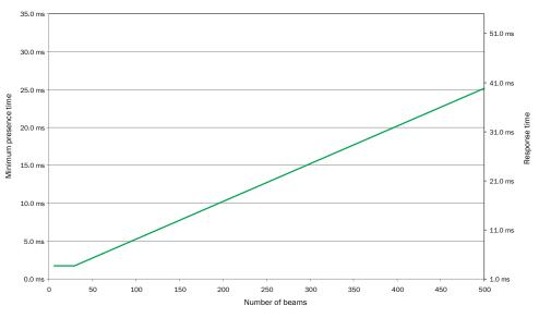
Figure 146: Graph, MLG-2 Pro response time and minimum presence time
