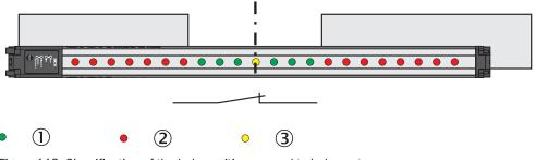
Figure 118: Classification of the hole position - equal to hole center
