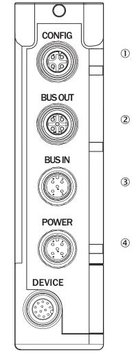
Figure 44: Fieldbus module connections
