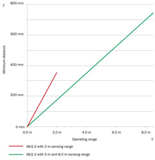
Figure 31: Graph, distances when light is in the same direction (XZ)
