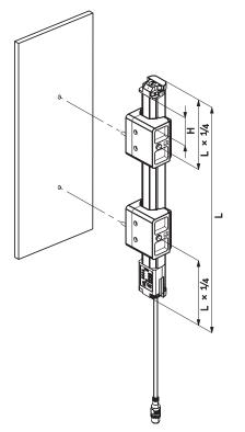
Figure 47: Alignment with the QuickFix bracket
