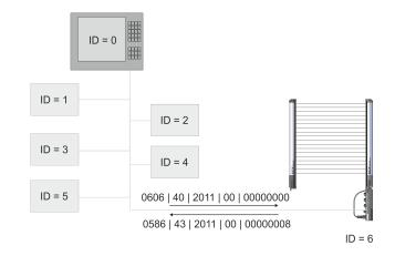
Figure 55: Example of a Receive SDO and a Transmit SDO
