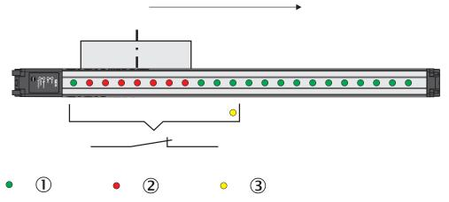
Figure 113: Classification of the object position – object center is smaller than or equal to n beam
