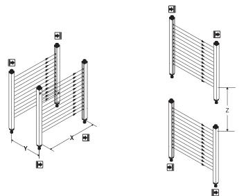
Figure 29: Distances when light is in the same direction
