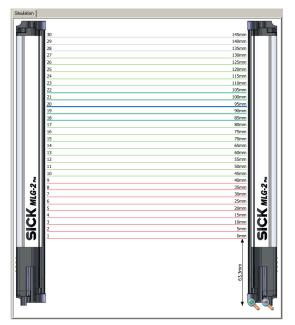
Figure 81: Detection area – Simulation
