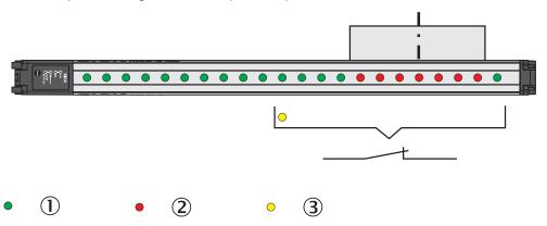
Figure 112: Classification of the object position – object center is greater than or equal to n beam
