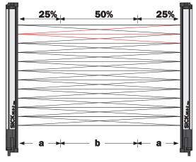
Figure 15: Cross-beam function
