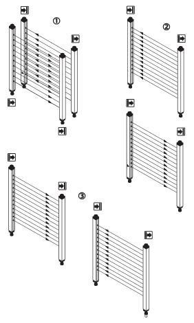
Figure 28: Placement with light in opposite directions
