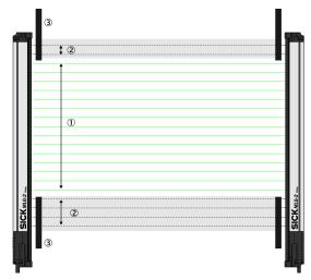
Figure 7: Detection area with beams blanked
