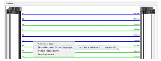
Figure 83: Using beams for object recognition
