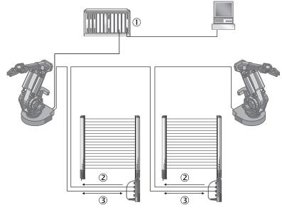
Figure 52: Example of a CANopen network in a line structure
