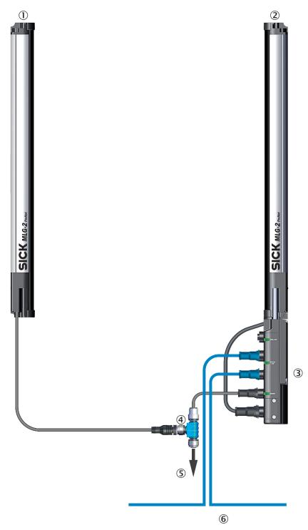
Figure 45: Connection with T-distributor
