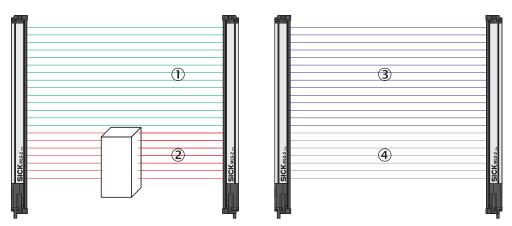
Figure 127: Example of the blanking of blocked beams
