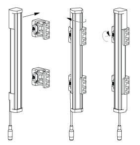
Figure 38: Inserting the MLG-2 in the FlexFix brackets
