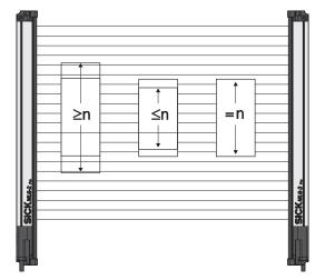
Figure 103: Object detection/object width
