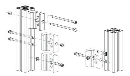
Figure 35: Mount QuickFix bracket to a profile frame
