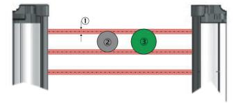
Figure 13: Minimum detectable object
