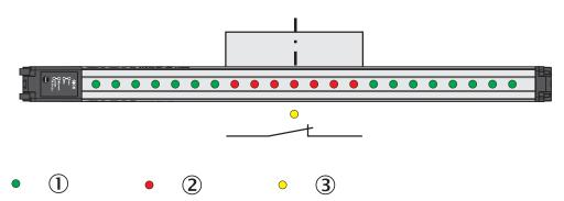
Figure 114: Classification of the object position - object center is equal to n beam
