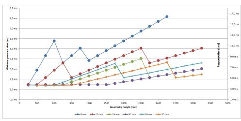
Figure 148: Response time and minimum presence time up to 3.5 m sensing range
