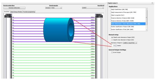
Figure 96: Example representation of the outer dimension
