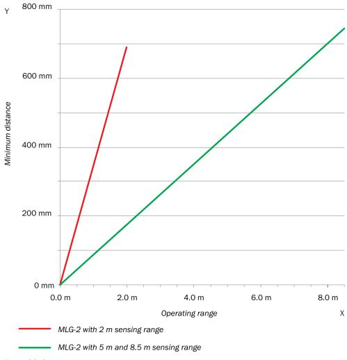
Figure 30: Graph, distances when light is in the same direction
