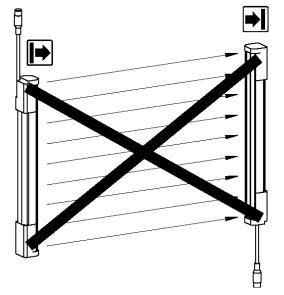
Figure 34: The sender and receiver are aligned incorrectly
