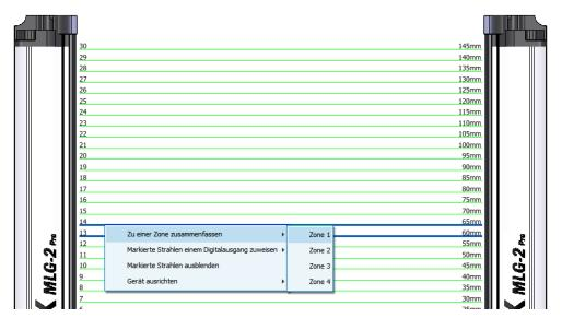
Figure 82: Combining beams into zones
