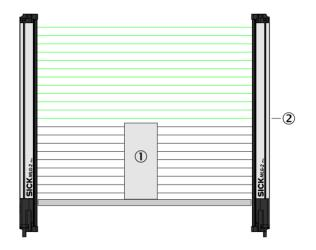
Figure 60: Beam function FBM
