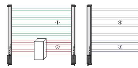
Figure 72: Example of blanking made beams
