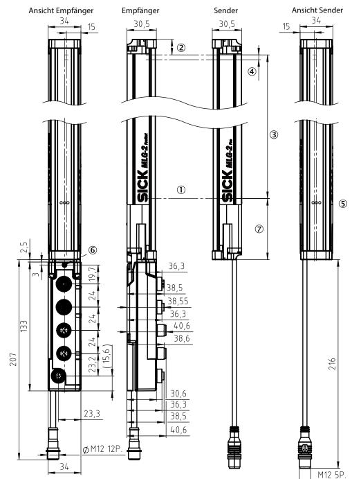
Figure 151: Dimensional drawing MLG-2 ProNet (mm)
