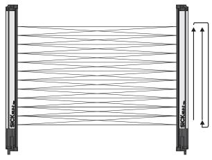
Figure 10: Cross-beam function
