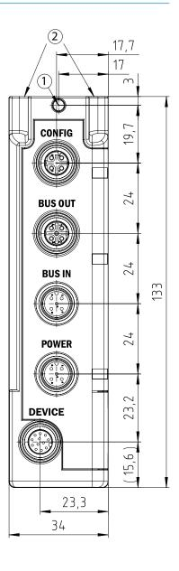
Figure 153: Dimensional drawing 2 MLG-2 fieldbus module
