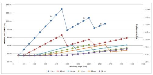
Figure 149: Response time and minimum presence time up to 8.5 m sensing range
