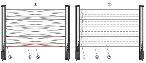
Figure 132: Left: "Cross beam switching", right: "Cross beam measuring"
