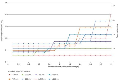
Figure 147: Response time and minimum presence time up to 2 m sensing range
