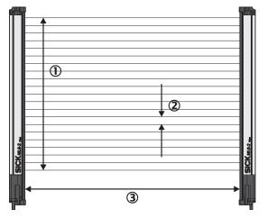
Figure 5: Detection area of the MLG-2
