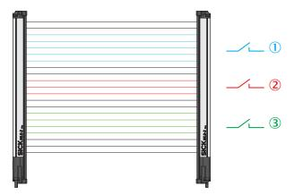
Figure 121: Measuring within zones
