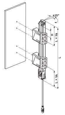
Figure 48: Alignment with the FlexFix bracket
