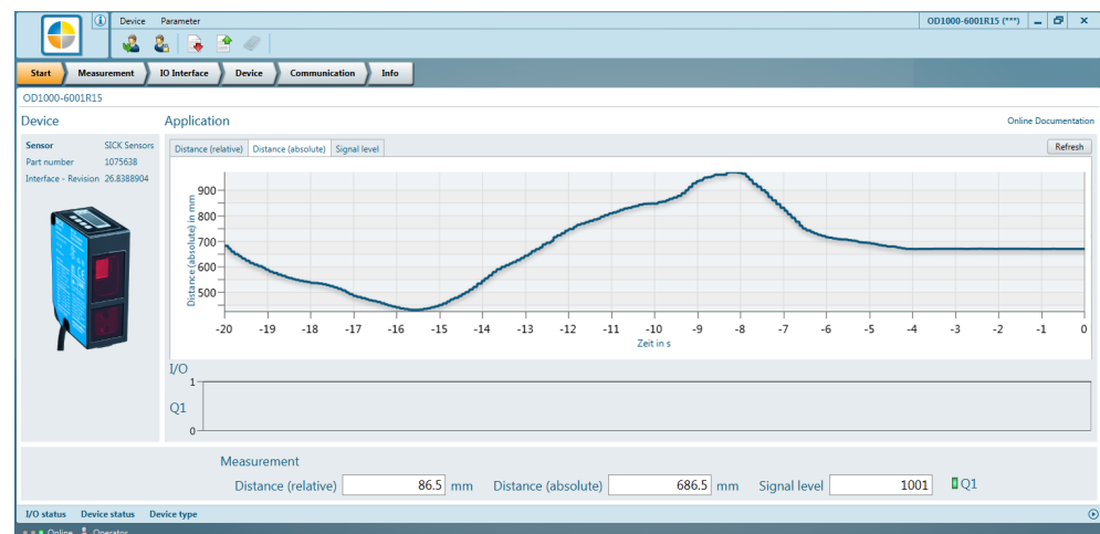
Figure 20: SOPAS ET start screen – visualization of the distance values and the output state
