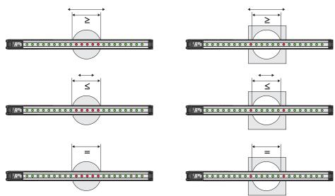
Figure 103: Measurement of the outside dimension
