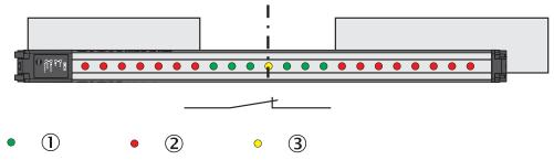
Figure 112: Classification of the hole position - equal to hole center
