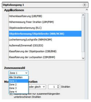
Figure 117: SOPAS ET - Assigning an application and zone to an output
