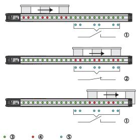
Figure 94: Object recognition, static
