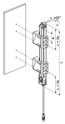
Figure 47: Alignment with the FlexFix bracket
