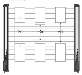
Figure 100: Hole detection/hole size
