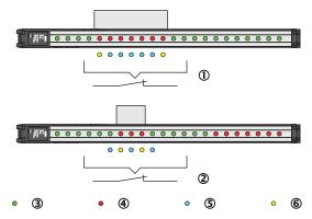
Figure 96: Object recognition with tolerance
