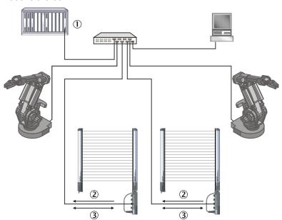
Figure 50: Example of a PROFINET network in a star structure
