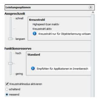
Figure 129: SOAPS ET - Activating cross beam measuring mode
