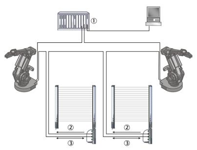
Figure 51: Example of a PROFINET network in a ring structure
