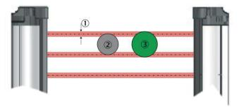
Figure 13: Minimum detectable object
