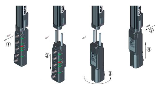
Figure 40: Turn the fieldbus module by 180°
