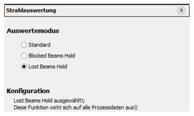
Figure 132: SOPAS ET - "Lost Beams Hold (LBH)" function
