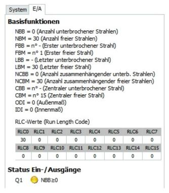
Figure 75: Basic functions and status of the output
