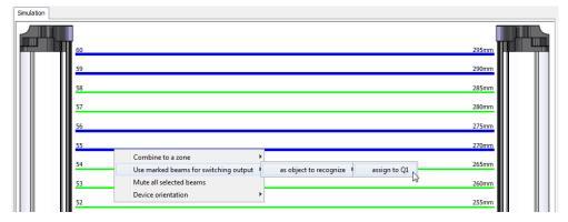
Figure 78: Using beams for object recognition
