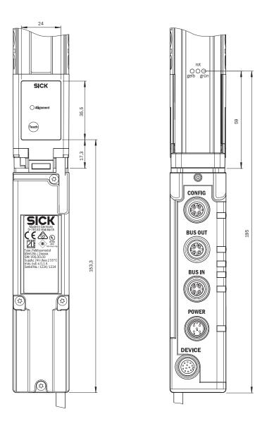
Figure 147: Dimensional drawing 1 MLG-2 fieldbus module
