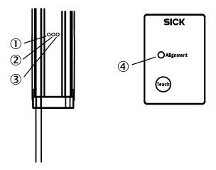
Figure 18: LEDs on the front and on the control panel
