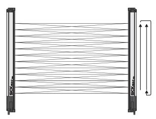
Figure 10: Cross-beam function
