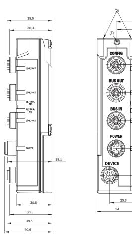
Figure 148: Dimensional drawing 2 MLG-2 fieldbus module
