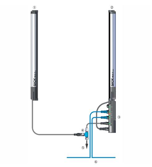
Figure 44: Connection with T-distributor
