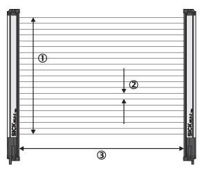
Figure 5: Detection area of the MLG-2
