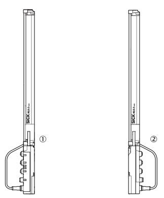
Figure 39: Mounting directions of the fieldbus module
