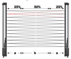
Figure 15: Cross-beam function
