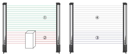
Figure 123: Example of blanking made beams
