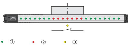
Figure 108: Classification of the object position – object center is equal to n beam
