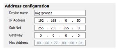
Figure 118: Address configuration for PROFINET
