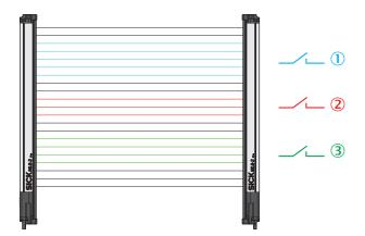
Figure 115: Measuring within zones
