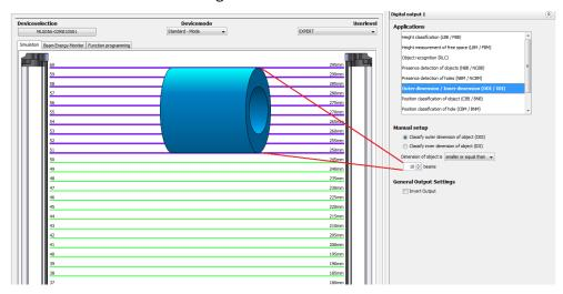
Figure 90: Example representation of the outer dimension
