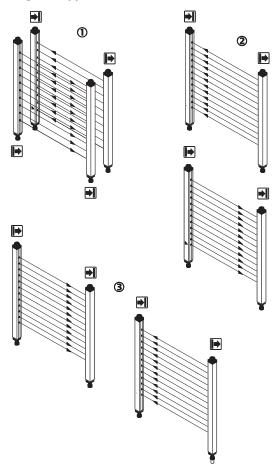
Figure 27: Placement with light in opposite directions
