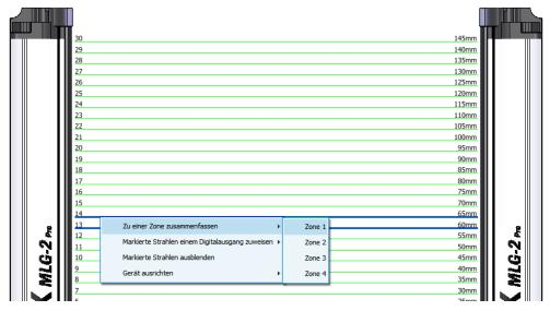
Figure 77: Combining beams into zones
