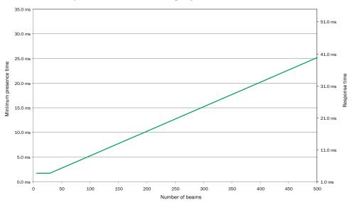
Figure 141: Graph, MLG-2 Pro response time and minimum presence time
