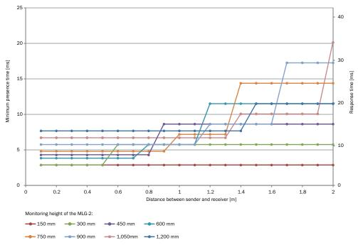
Figure 142: Response time and minimum presence time up to 2 m sensing range
