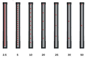
Figure 6: Schematic depiction of available beam separations (mm)
