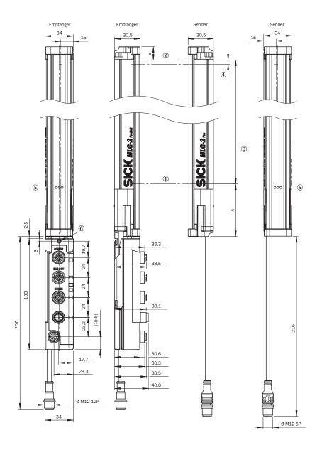
Figure 146: Dimensional drawing MLG-2 ProNet (mm)
