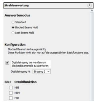
Figure 131: SOPAS ET - "Blocked Beams Hold (BBH)" function
