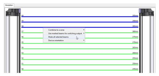
Figure 81: Blanking beams
