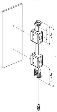
Figure 46: Alignment with the QuickFix bracket
