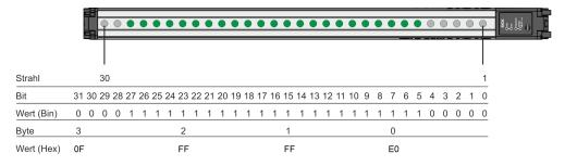
Figure 68: Bit-coded beam mask for an MLG-2, with 30 beams
