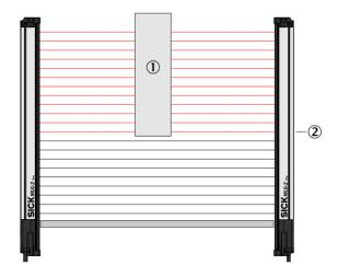
Figure 54: Beam function FBB
