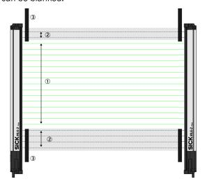
Figure 7: Detection area with beams blanked
