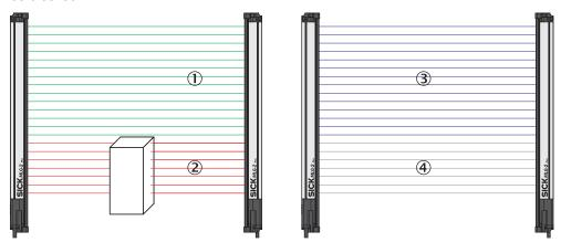
Figure 122: Example of the blanking of blocked beams
