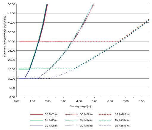
Figure 145: Minimum detectable absorption required for devices with  $2\,\mathrm{m}$ ,  $5\,\mathrm{m}$  and  $8.5\,\mathrm{m}$  sensing range
