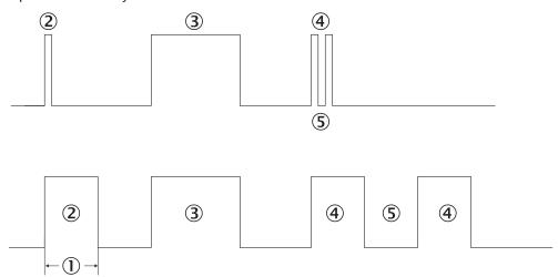
Figure 114: Examples of the effect of a configured minimum pulse width
