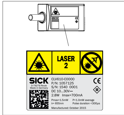
Installation site and design of the combination of black and yellow laser warning label and type label with laser performance data.
