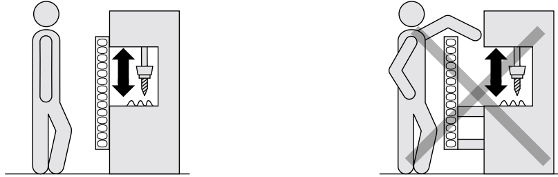
Figure 6: Representation of the accessibility of electro-sensitive protective device by reaching over. Left: Protective field that cannot be reached over. Right: Protective field that can be reached over.
