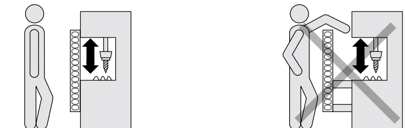
Figure 8: Representation of the accessibility of electro-sensitive protective device by reaching over. Left: Protective field that cannot be reached over. Right: Protective field that can be reached over.
