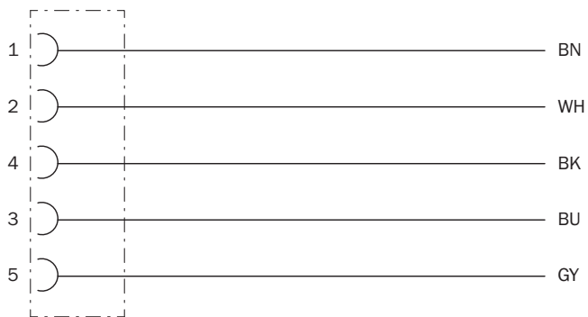
Contact assignment of the M12 female connector
