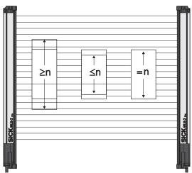
Figure 97: Object detection/object width
