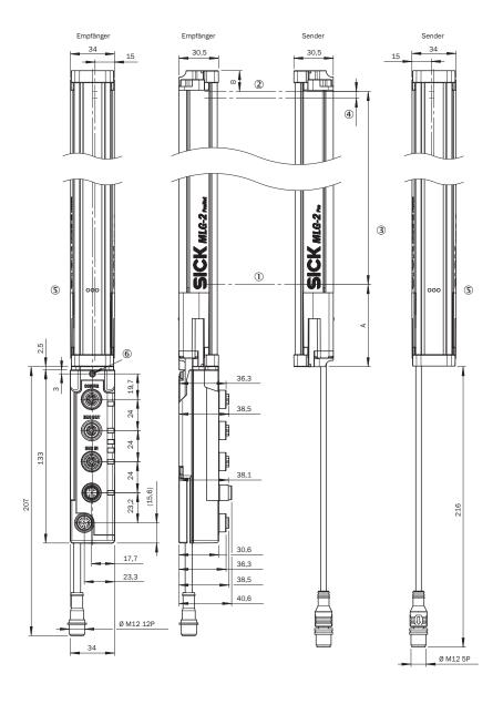
Figure 146: Dimensional drawing MLG-2 ProNet (mm)
