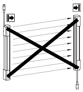
Figure 33: The sender and receiver are aligned incorrectly
