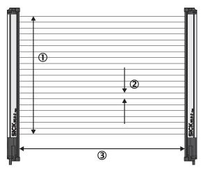
Figure 5: Detection area of the MLG-2
