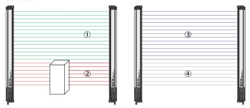
Figure 66: Example of the blanking of blocked beams
