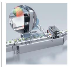
Figure 21: Start and end detection
