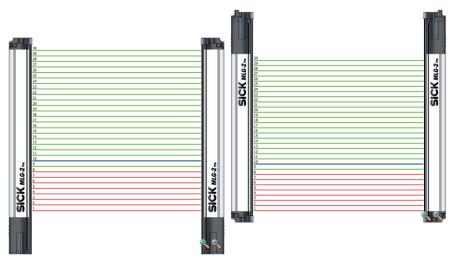
Figure 89: Beam numbering
