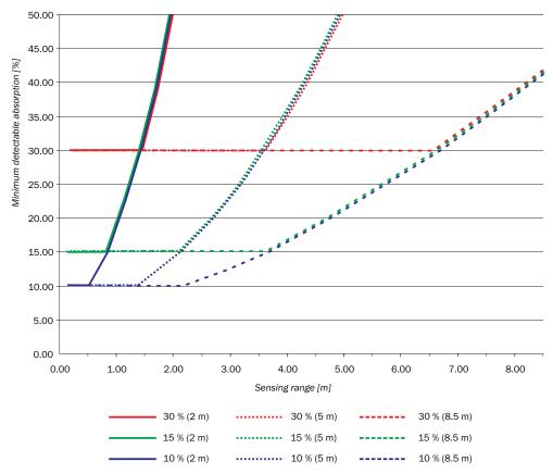
Figure 145: Minimum detectable absorption required for devices with 2 m, 5 m and 8.5 m sensing range
