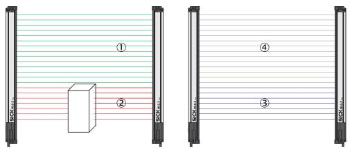
Figure 123: Example of blanking made beams
