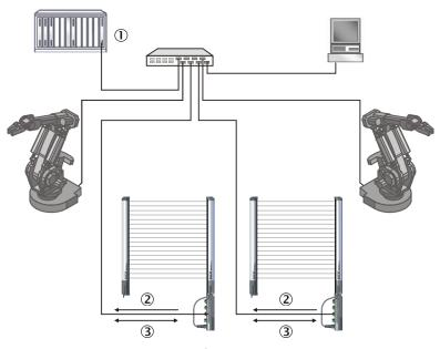
Figure 50: Example of an EtherCAT® network in a star structure
