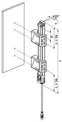
Figure 47: Alignment with the FlexFix bracket
