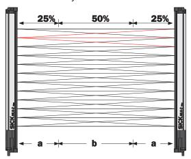
Figure 15: Cross-beam function
