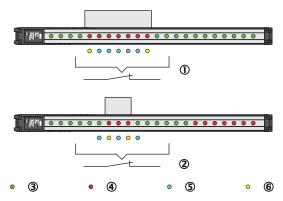
Figure 96: Object recognition with tolerance
