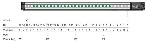
Figure 68: Bit-coded beam mask for an MLG-2, with 30 beams
