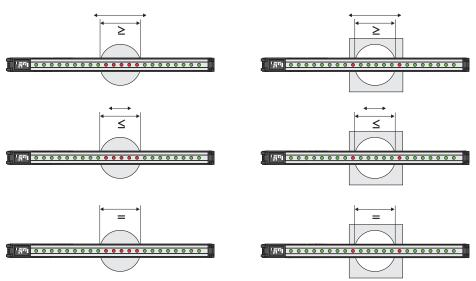
Figure 103: Measurement of the outside dimension
