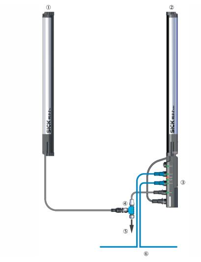
Figure 44: Connection with T-distributor
