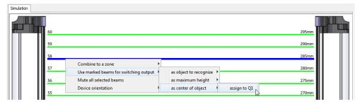
Figure 80: Using beams to classify the object position
