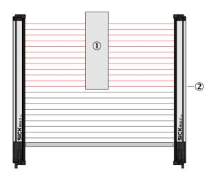
Figure 54: Beam function FBB
