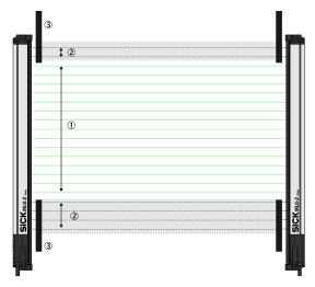
Figure 7: Detection area with beams blanked
