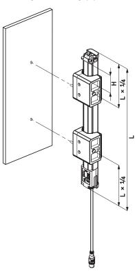
Figure 46: Alignment with the QuickFix bracket
