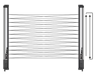
Figure 10: Cross-beam function
