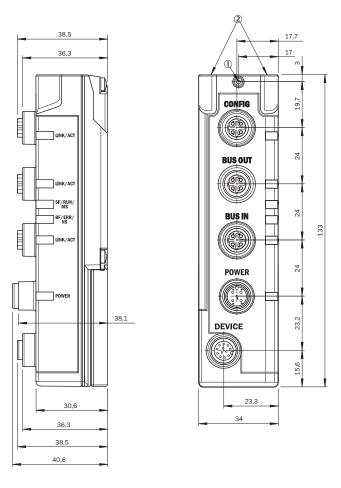
Figure 148: Dimensional drawing 2 MLG-2 fieldbus module
