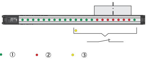
Figure 106: Classification of the object position – object center is greater than or equal to n beam
