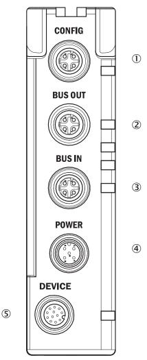
Figure 43: Fieldbus module connections
