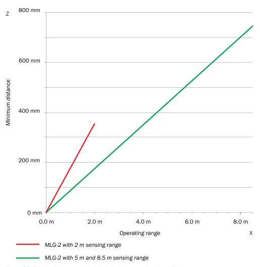
Figure 30: Graph, distances when light is in the same direction (XZ)
