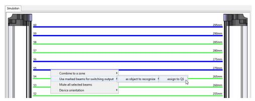
Figure 78: Using beams for object recognition
