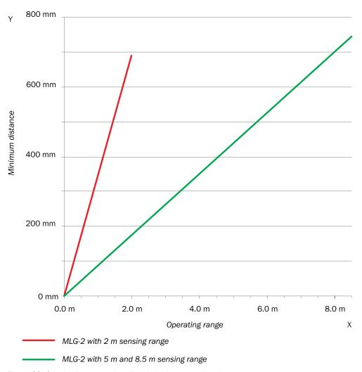
Figure 29: Graph, distances when light is in the same direction
