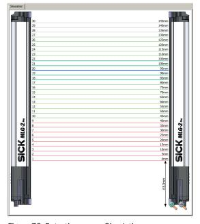
Figure 76: Detection area - Simulation
