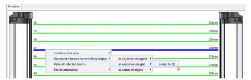
Figure 79: Using beams for height classification
