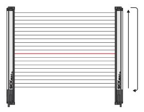
Figure 8: Standard scan method
