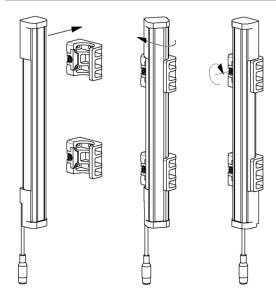
Figure 37: Inserting the MLG-2 in the FlexFix brackets
