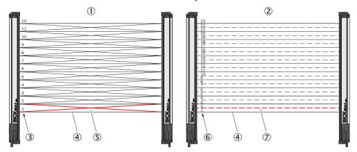
Figure 127: Left: "Cross beam switching", right: "Cross beam measuring"
