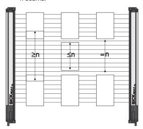
Figure 100: Hole detection/hole size
