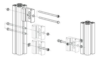
Figure 34: Mount QuickFix bracket to a profile frame
