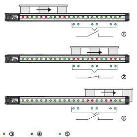
Figure 94: Object recognition, static
