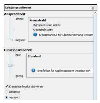
Figure 129: SOAPS ET - Activating cross beam measuring mode
