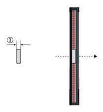
Figure 14: Minimum detectable object length
