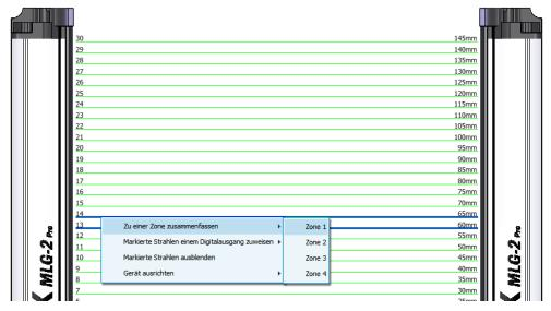
Figure 77: Combining beams into zones
