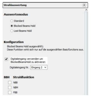
Figure 131: SOPAS ET - "Blocked Beams Hold (BBH)" function
