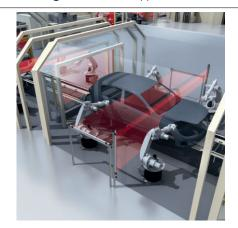
Figure 26: Contour measurement
