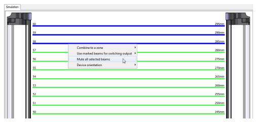
Figure 81: Blanking beams
