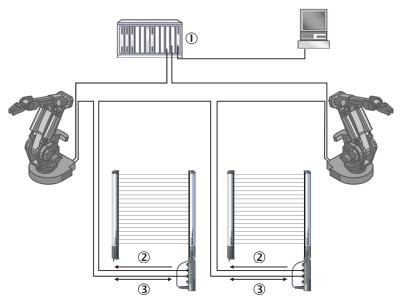
Figure 51: Example of an EtherCAT® network in a ring structure
