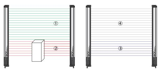
Figure 67: Example of blanking made beams
