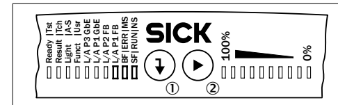
Fig. 12: LED status indicators, function buttons and bar graph display
