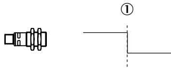
Fig. 8: Teach-in the switching point – method A
