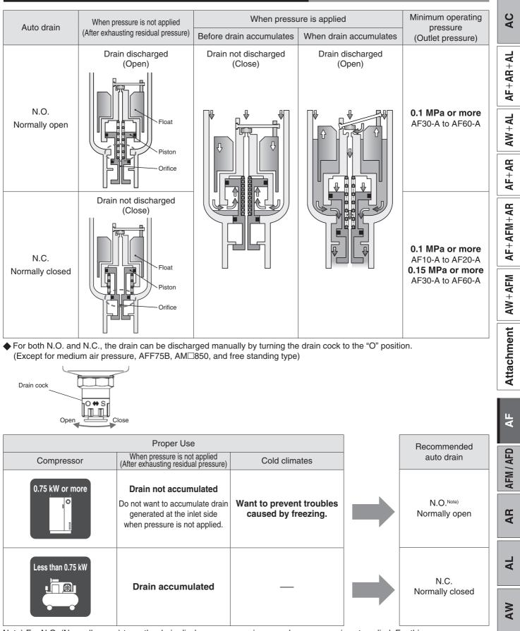
**Operating State and Proper Use of Float Type Auto Drain**
